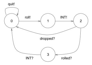
Figure 2. Finite state machine representing the DIE protocol
